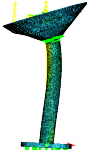
Figure 1 - Resonance of a water tower - numerical model
